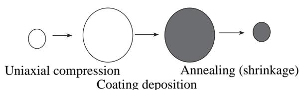
**Fig. 1.** Schematic representation of the experimental procedure for the visualization of structural rearrangements during temperature-induced shrinkage of the polymer sample after its deformation via uniaxial compression.
