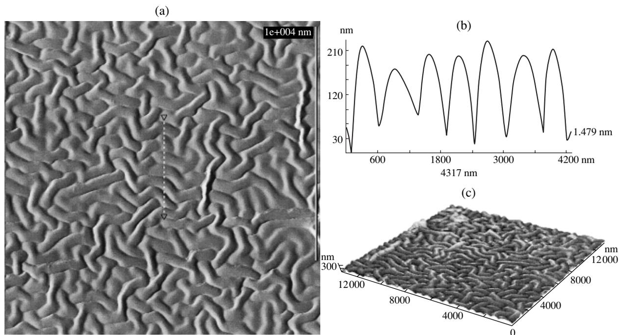
**Fig. 2.** (a) AFM image, (b) surface profilogram, and (c) 3D reconstruction of AFM image of the biaxially oriented PET sample coated with a thin (15 nm) platinum layer after its annealing at 210°C.
