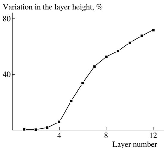
**Fig. 5.** Uniaxial compression strain of individual layers of PMMA (the initial thickness of each layer is 1 mm) vs. their location with respect to the compressing surface. The total uniaxial compression strain of the multilayered sample is equal to 30%.
