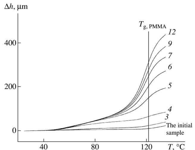
**Fig. 6.** Absolute changes in the height of individual PMMA layers after deformation of the multilayered sample by 30% at room temperature. Numbers at curves correspond to the position of each layer with respect to the compressing surface.
