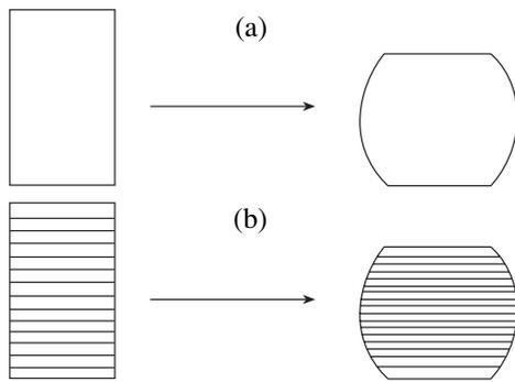
**Fig. 4.** Schematic representation of uniaxial compression tests of the polymer sample, which was (a) described in [5, 6] and (b) used in this work.
