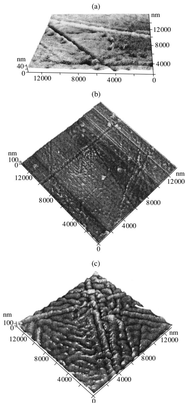
**Fig. 3.** AFM images of PMMA samples after their uniaxial compression by 20% and annealing at (a) 50, (b) 70, and (c) 90°C after deposition of thin (15 nm) platinum coating.
