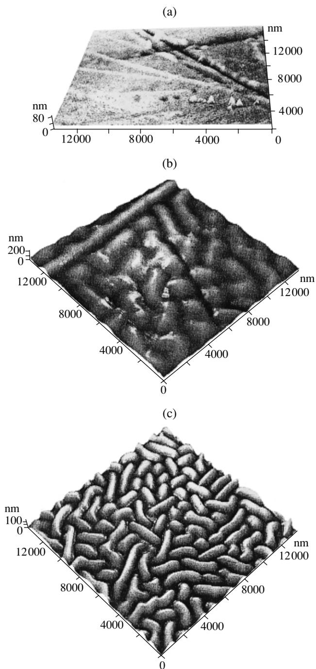
**Fig. 7.** AFM images of individual layers after deformation of the multilayered PMMA sample by 30%. The individual layers were coated with a thin (15 nm) platinum coating and annealed at 130°C. Shrinkage: (a) 1.7, (b) 20.8, and (c) 45%.
