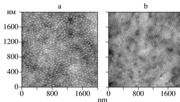
**Fig. 3.** AFM images of the SMAS films for [PS] : [PMA] = 1 : 2 (domain structure, left) and [PS] : [PMA] = 1 : 1 (lamellar structure, right).
