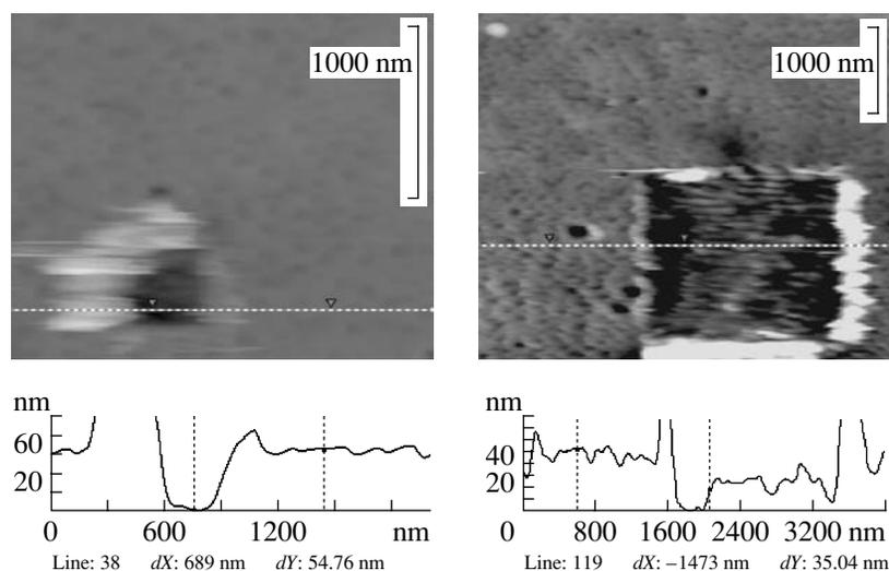
**Fig. 1.** AFM images of the SBS (left) and SMAS films (right) with the areas from which the polymer is removed. The cross section of the surface is shown at the bottom.
