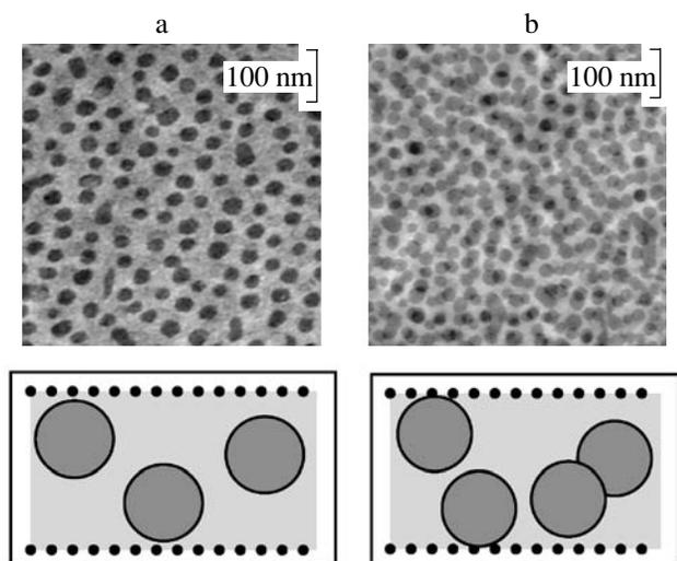
**Fig. 4.** TEM images of different areas of the SBS film (top) and the theoretical models of domain arrangement (bottom).
