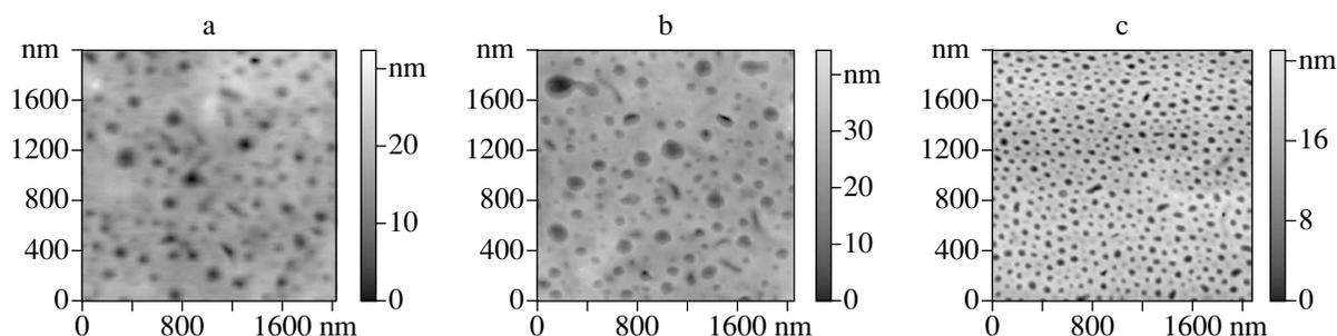
**Fig. 2.** AFM images of the SBS films obtained under different conditions: (a) rapid evaporation of the solvent, (b) slow evaporation of the solvent in the saturated vapor of toluene, and (c) slow evaporation of the solvent followed by annealing at 110°C for 2 h.
